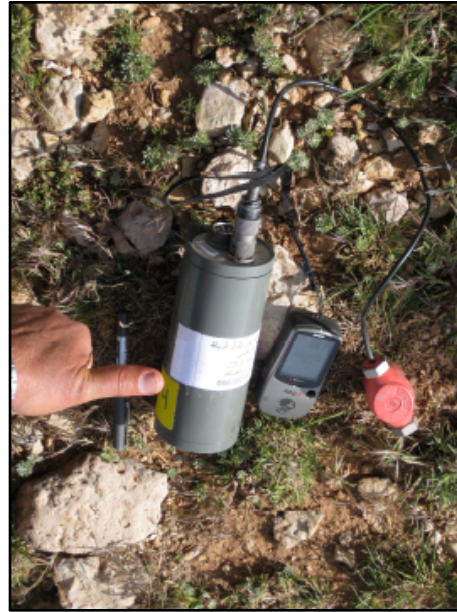
Geophone that will be used in iMUSH.
