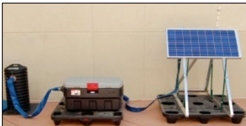
Equipment used in an iMUSH passive-source seismic station. On the left is the seismometer, data recorder and battery housing in the center and the solar panel on the right. Image courtesy of the University of Washington.
